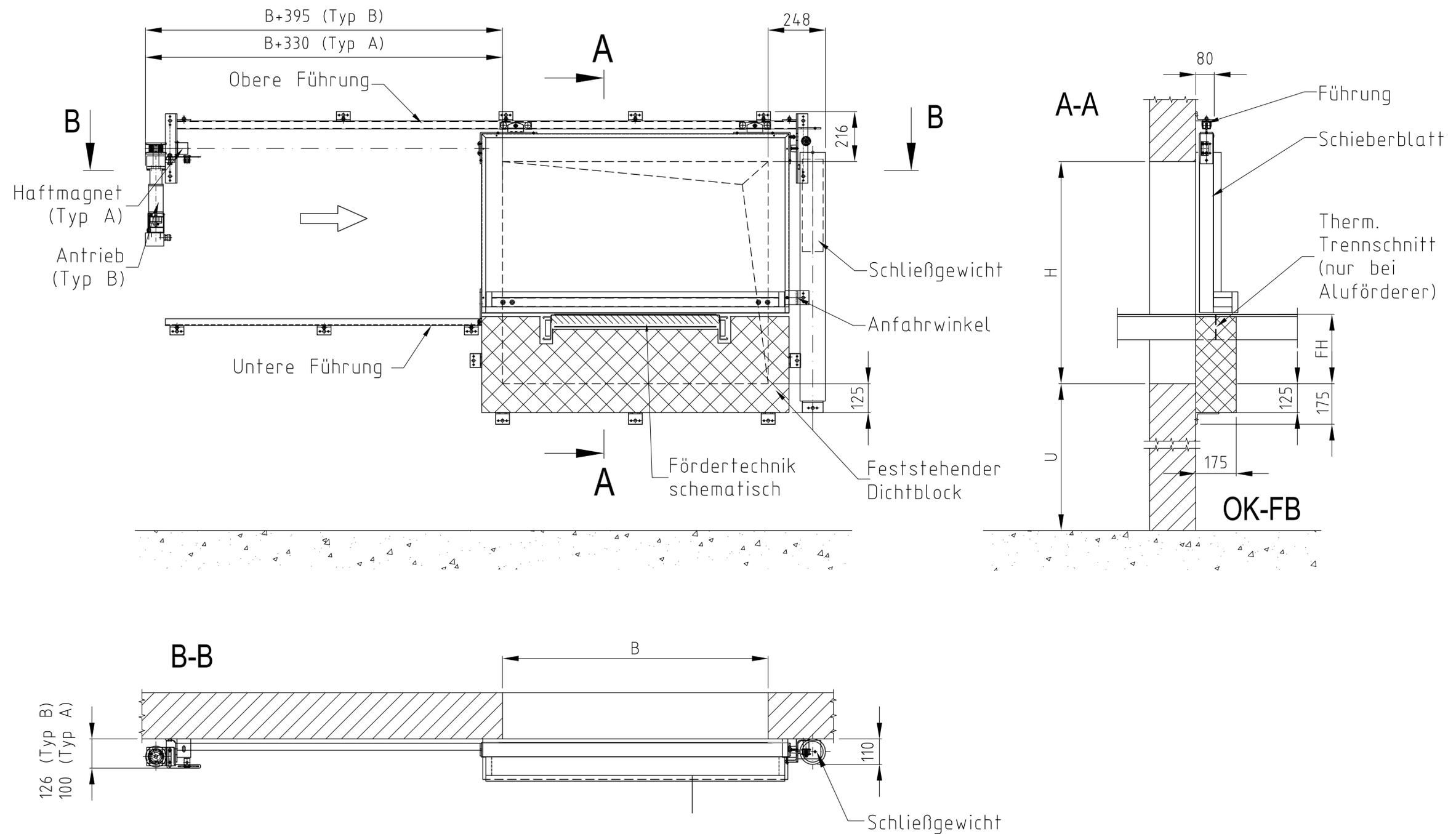
$B_{max} \times H_{max} = 3750 \times 3750$  (max. lichte Fläche  $9,38m^2$ )
